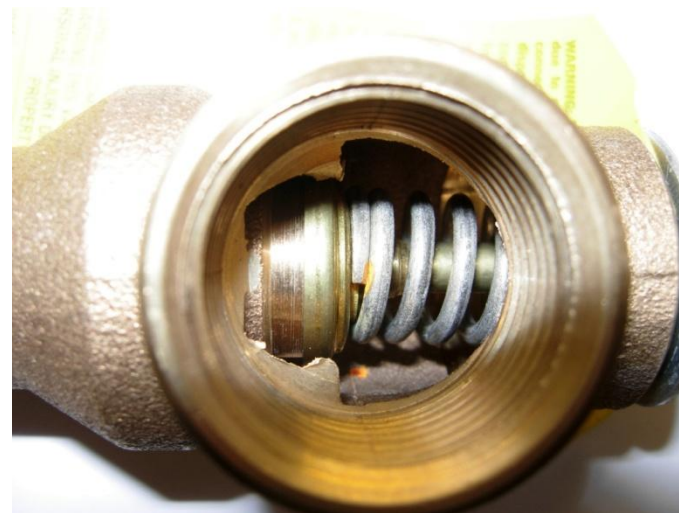
New TPR valve has solid metal and no buildup or corrosion
