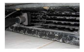
4. Use a special coil cleaning brush to remove dust farther back inside the coils.
