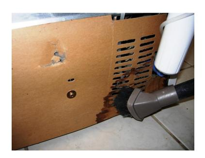
8. Use the vacuum cleaner with brush attachment to clean both inside and outside the kickplate.
