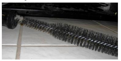
Reasonable force should be used with the brush; avoid jabbing or violent motion which might damage the coils.
